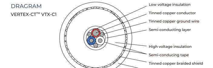
Red Insulation is 1.5mm<sup>2</sup>, White & Blue Insulation is 0.5mm<sup>2</sup>, Ground wire is 1.5mm<sup>2</sup>.
