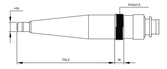
The VERTEX-N<sup>TM</sup> VC-N1 connector can be adapted to the following types of cables VERTEX-R<sup>TM</sup> VTX-R3 (100kVDC) VERTEX-N<sup>TM</sup> VTX-N1(160kVDC)
