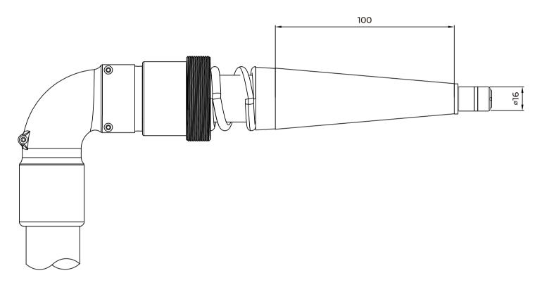
The VERTEX-N<sup>TM</sup> VC-N190SL connector can be adapted to the following types of cables VERTEX-R<sup>TM</sup> VTX-R3 (100kVDC) VERTEX-N<sup>TM</sup> VTX-N1(160kVDC) VERTEX-N<sup>TM</sup> VTX-N2(250kVDC)
