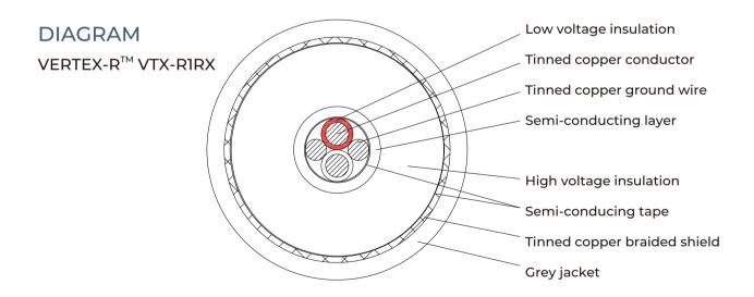
White and red insulation is 1.5mm<sup>2</sup>, The ground wire is 1.8mm<sup>2</sup>.
